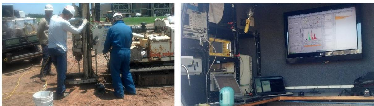
Figure 2. The screening performed by pushing probe into the soil, while the LIF system displayed *n* real-time LNAPL fluorescence occurrence
